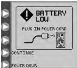
Figure 32 Battery Low error screen. Indicates that the battery must be recharged immediately.
