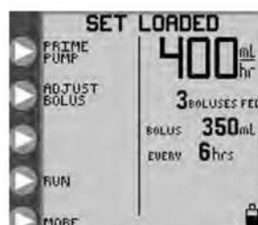
Figure 7C. Opening menu for Intermittent Feed mode with a feed-only set.
