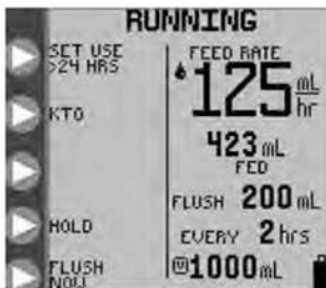
Figure 34. Running screen with the > 24 HRS of Pump Set Usage indicator in upper left of the screen.
