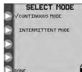
Figure 10B. SELECT MODE menu for continuous or intermittent mode selection.
